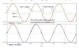
Figure 8: Signals in combined ADCs of Fig. 7, with audible "glitches" in the summed signal [10]
